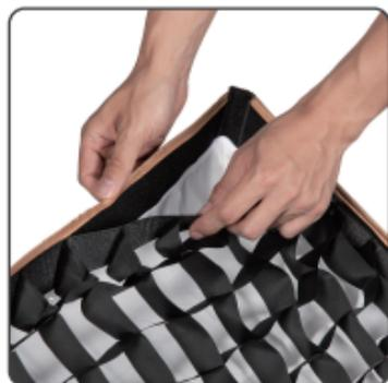
4. Attach the honeycomb grid to the edge of the softbox with velcro.
