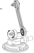
② Install the extension arm and shock absorber support 连接延长杆与减震臂
