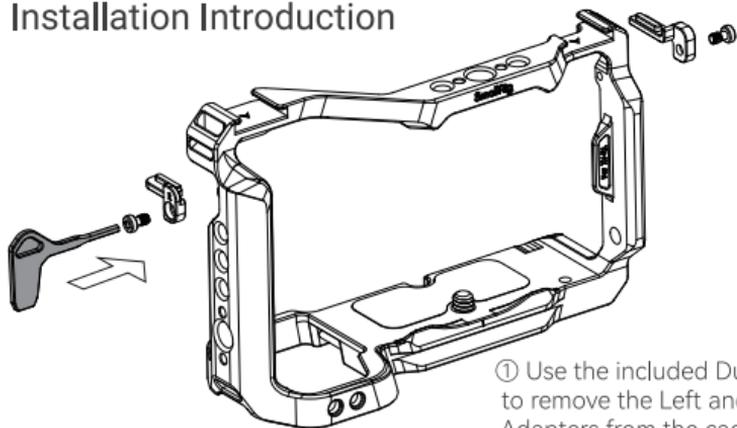
① Use the included Dual-Head Wrench to remove the Left and Right Side Lock Adapters from the cage.
