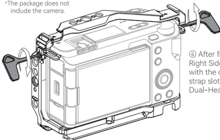
④ After fixing the Left and Right Side Lock Adapters with the camera shoulder strap slots, lock them by the Dual-Head Wrench.
