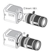
2. Installing Gobo: Place the desired gobo into the clip, then insert the clip into the slot.
