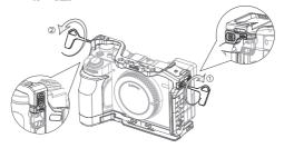
Step 4: Use the double head wrench to secure the cage by tightening the 1/4"-20 screw.
