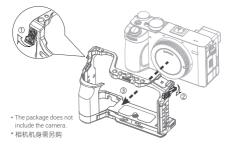
Step 3: Fix the locating blocks to the camera's triangular ring, then use the double head wrench to tighten the M3 screw on both sides of the cage.
