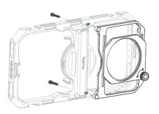
② Extended the filters: align the 67mm threaded filter with the filter adapter ring and thread it to complete the installation. This product is suitable for the standard 67mm threaded filter on the market, and the SmallRig 67mm magnetic filter series (with the switch adapter from magnetic to threaded).
