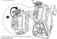
(4) Use the double head wrench to move the M4 screw on the bottom of the plate to the top left corner of the plate, then secure the cage by tightening.
