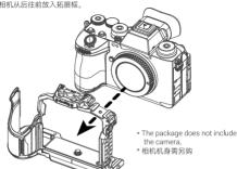
(2) Use the double head wrench to secure the cage by tightening the 1/4"-20 screw. 通过双头扳手拧紧底部1/4"-20螺丝、锁紧固定拓展框。
