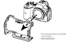
(3) Secure the cage and camera strap slots by tightening two locatirng blocks on the sides of the cage.
