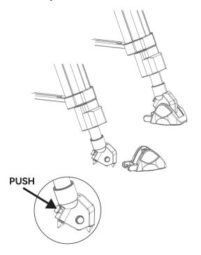
To use the nail, press the button, and remove the rubber foot from the nail.
