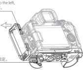
(2) Slide the Locating block into the camera strap slot from left to right, then fix it by tightening the screws. 将定位压块从左往右滑进相机肩带槽、通过锁紧螺丝固定。
