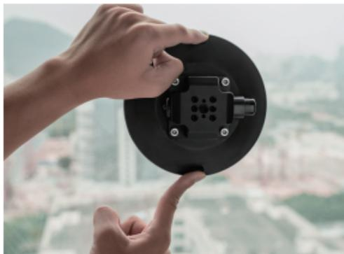
**08** When disassembling, simultaneously pull up on the handle until the suction cup unlocks.
