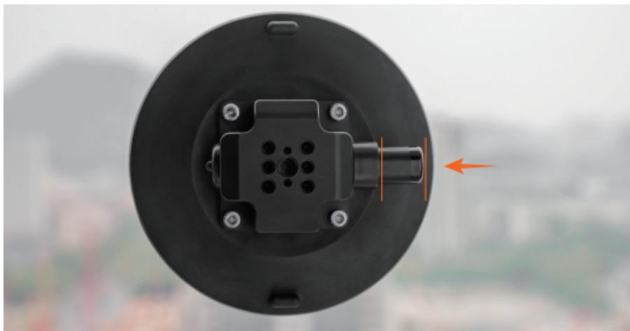
**05** When the white marking line on the air pump is only partially retracted, it indicates that the suction is incomplete. Please continue pressing the air pump until it is tightly locked in place.
