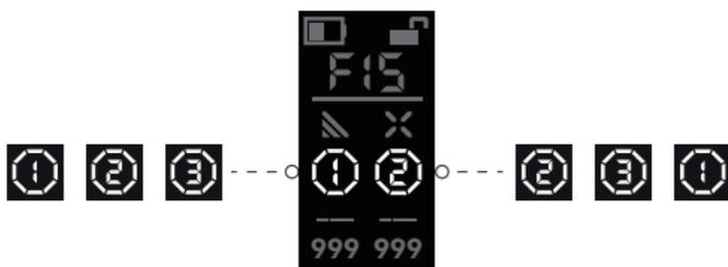
Electronic Controller Module Handgrip Mode: Press and hold ▲ to activate the motor number; click ▲ / ▼ to adjust the number; press and hold ▲ to exit.
