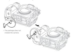
Step3: Use the Dual Head Wrench to loosen the screw that fixes the locating block, but do not unscrew it completely. Align and tighten it close to the camera strap groove
