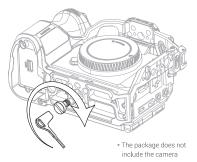
Step2: Use the Dual Head Wrench to remove the M4 screws at the bottom of the cage, align and tighten the M4 screws to the corresponding positions to secure the cage
