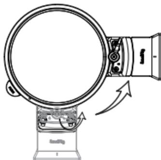
2. Install the connecting plate: Align the connecting plate with the two M4 screws at the bottom of the mounting plate and use the allen wrench to lock it, and please do not lock it completely here.
