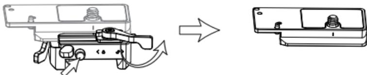
2. Install the quick release plate: Align the quick release plate with the 1/4"-20 threaded holes and locating holes at the bottom of the camera, then lock and fix it by the dual-head wrench ⑪ at the bottom of the connecting plate. (\*Please ignore this step if using camera cages)
