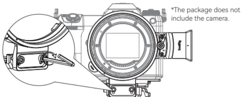
5. Rotate the lens ring 90° clockwise, then lock the horizontal-to-vertical locking lever ③.
