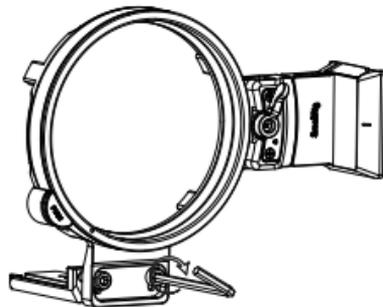
3. Install the lens ring: Unlock the lens ring locking lever ⑮, slide the lens ring connecting plate into the slot hole under the baseplate and then lock the lens ring lever ⑮.
