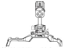
$\label{eq:Step 3: Push the lever to the right to secure the handle.}$
