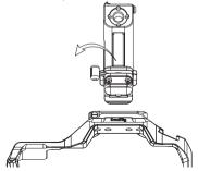
Step 2: Align and press the NATO clamp into the NATO Rail to install.
