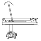
**Step 2:** After adjusting to the suitable position, tighten the two M5 screws to secure the handle adapter.
