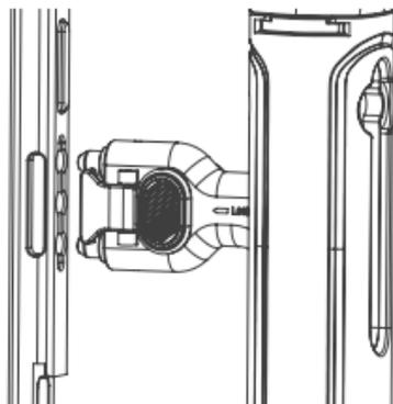
(3) **Attach the Phone:** Press the unlock button on the left side of the cage, open the cover, and slowly slide the phone into the cage body. Then close and press the upper cover until you hear a "click" sound, indicating that the upper cover and lower body are locked.
