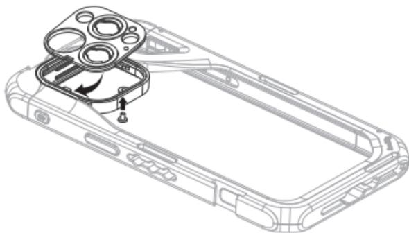
**(5) Install Filters:** Install a filter adapter ring on the back panel to use external filters. Filters and M-mount filter adapters need to be purchased separately.
