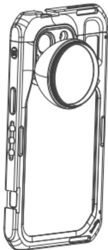
**Replace the Lens Panel:** Remove the 1/4"-20 screw inside the cage with a screwdriver and remove the lens panel diagonally to the right. As shown in the figure below, snap the back panel diagonally to the left into the slot of the cage, then insert the panel into the cage body, and finally tighten the 1/4"-20 screw from the inside of the cage.
